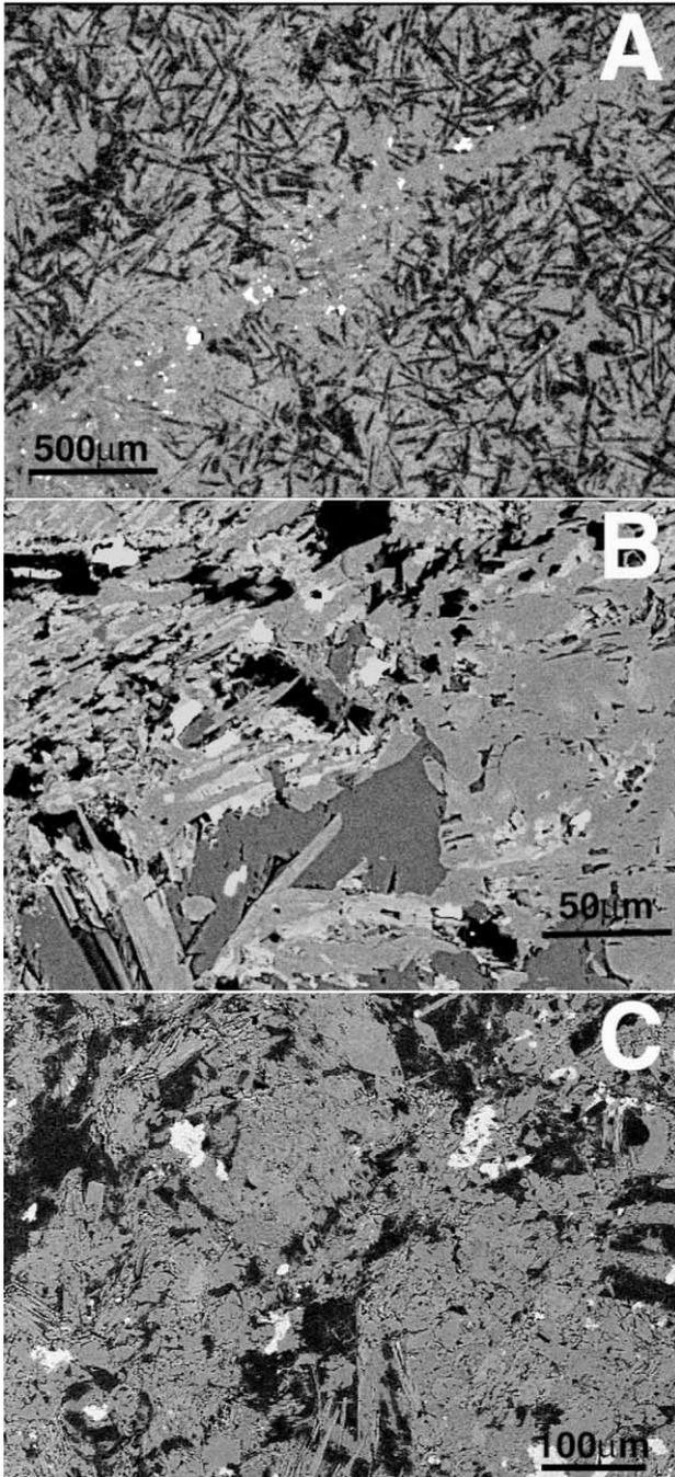
Fig. 8. An SEM reflection image of (A and B) Considerable creek and (C) Beasley river basalts: (A) a diagonal array of white grains are pyrite and dark acicular crystals are albite; (B) gray euhedral crystals are calcite; (C) white grains are titanite and the dark area are quartz.
