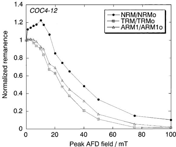
Fig. 11. Alternating field demagnetization of NRM, TRM and ARM (before heating) during the Shaw method shown in Fig. 10.
