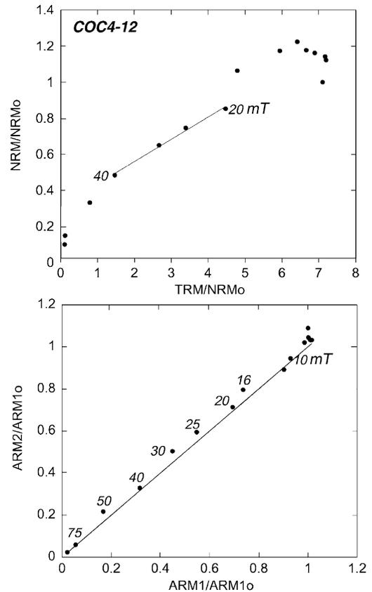
Fig. 10. Result of Shaw method for Considerable creek pillow basalt. Top: TRM–NRM plot with the linear fit used to determine the paleointensity. Numbers indicate the peak demagnetization field (in mT). Bottom: ARM checks before (ARM1) and after (ARM2) heating. The line indicates a slope of 1.
