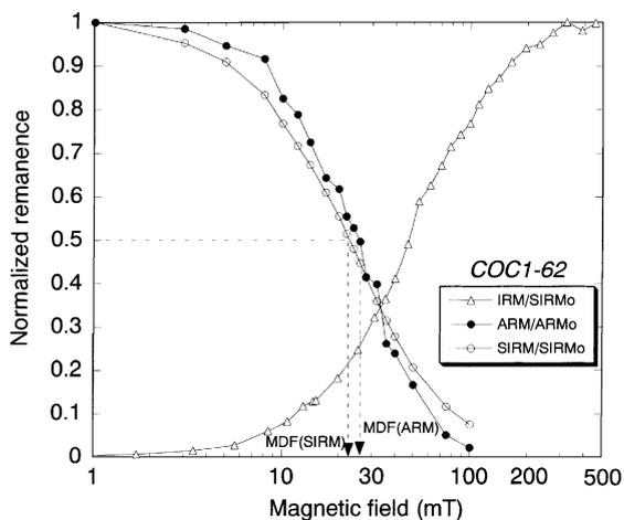
Fig. 6. IRM acquisition and alternating field demagnetization of ARM and SIRM of Considerable creek pillow basalt. The arrows indicate the mean destructive field (MDF) of ARM and SIRM.
