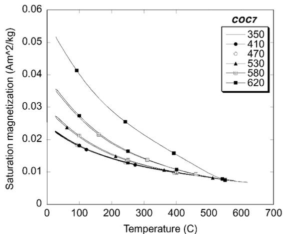
Fig. 7. Temperature dependence of saturation magnetization under a magnetic field of 100 mT for Considerable creek pillow basalt. The numbers indicate the maximum temperature (in  $^\circ\text{C}$ ) for each temperature loop.
