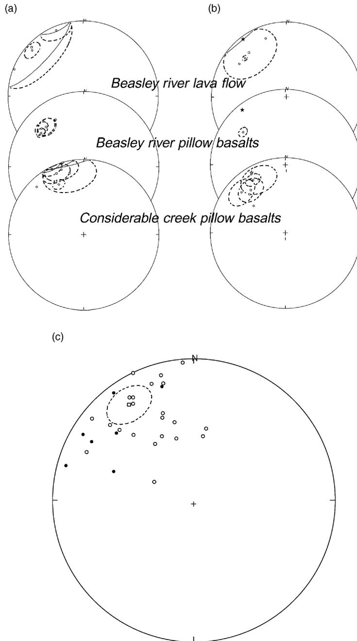
Fig. 3. Equal area plot of the paleomagnetic directions with confidence limits ( $\alpha_{95}$ ). Open (solid) marks indicate upward (downward) directions. Each circles represent the mean direction for each hand sample (cubic specimen for BIFs), squares represent the site mean direction: (a) mid-temperature components (in situ); (b) high-temperature components (in situ). Stars indicate the bedding corrected site mean direction. (c) Mid-temperature components (in situ) of the BIFs.
