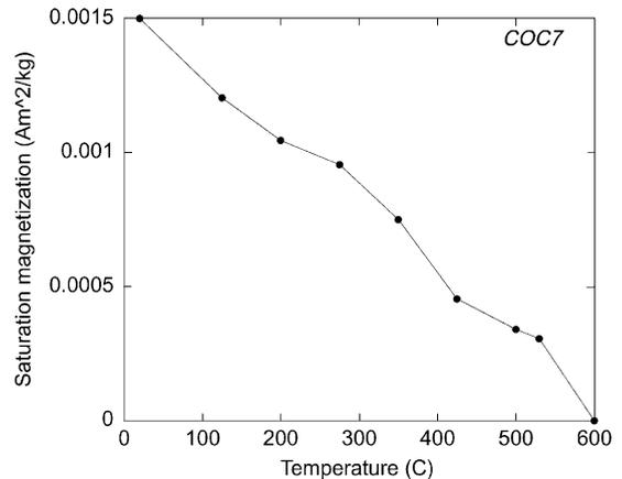
Fig. 5. Temperature dependence of saturation magnetization of ferromagnetic component determined from hysteresis curve. Specimen is the same as that used in Fig. 4.
