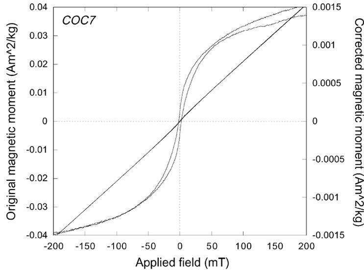
Fig. 4. An example of a hysteresis measurement for Considerable creek pillow basalt. Both the original data showing the dominance of paramagnetic linear component and the corrected data after subtracting the linear component are shown.
