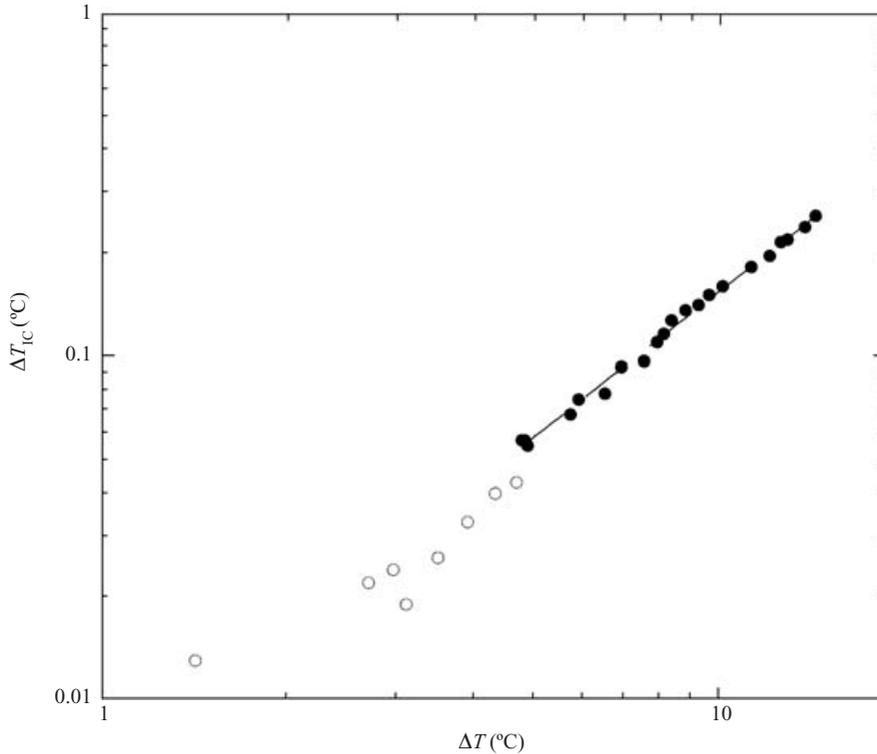
FIGURE 4. Relation between the imposed temperature difference across the shell  $\Delta T$ , and the temperature rise of the circulating water through the inner sphere  $\Delta T_{IC}$ . Data points in solid circles are used to obtain a power-law fit of  $\Delta T_{IC} = 0.006\Delta T^{1.41 \pm 0.02}$  (correlation coefficient 0.997).
